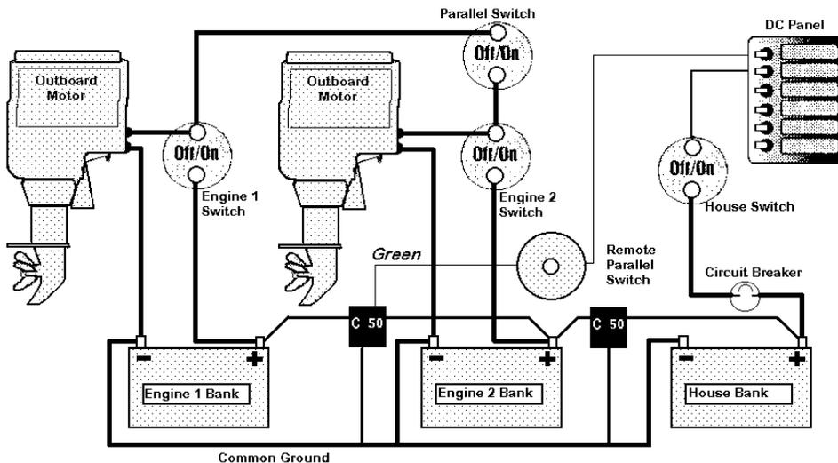
example there are twin engines, each with their own starting battery, and one house bank for auxiliary loads. Either engine can be started from either starting battery, or both in parallel. A remote parallel switch or push button can be located on the control panel to be used for assistance in an emergency. If any engine is running, all batteries will be charged.
