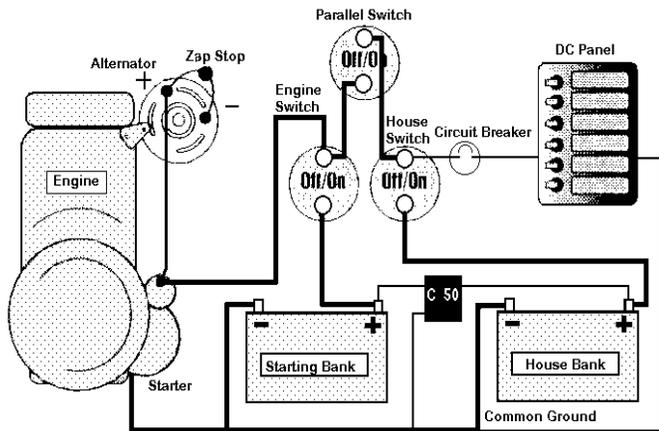
if the alternator output is accessible, is to remove it from the starter circuit and connect it directly to the house battery positive. The starting battery will now be charged through the combiner.
