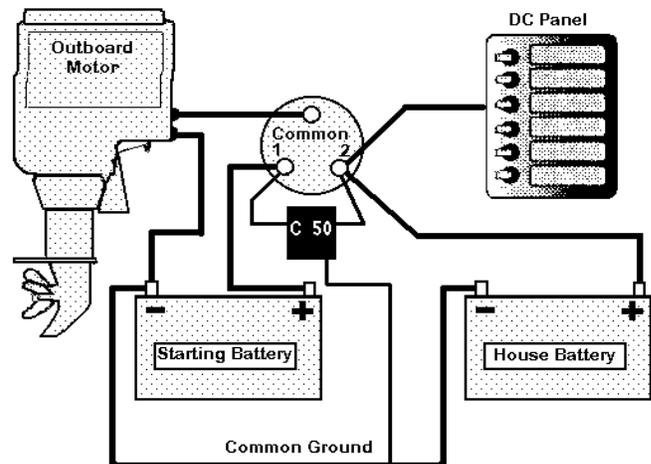
supplied from the starting battery in position 1 but battery 2 or both can be selected in an emergency. In all cases, both batteries are being charged when the engine is running.
